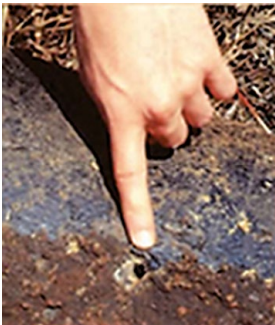
Typical perforation of a sewage system that is insufficiently protected against stray current.
